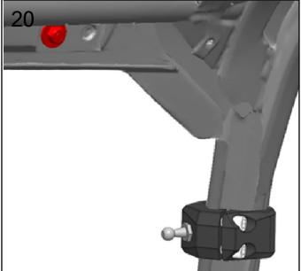
On the back side use one more **M8 Washer** followed by a **M8 Nylon Lock Nut.** Tighten and repeat for driver side.
