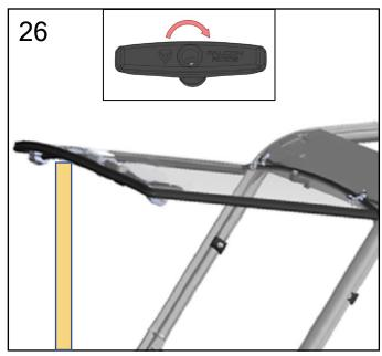
Twist the **T Handle** to open the windshield and lift it until it is parallel with the ground. Have a helper (or stick) hold the windshield in this position. You will need it to be open while you do the next few steps.
