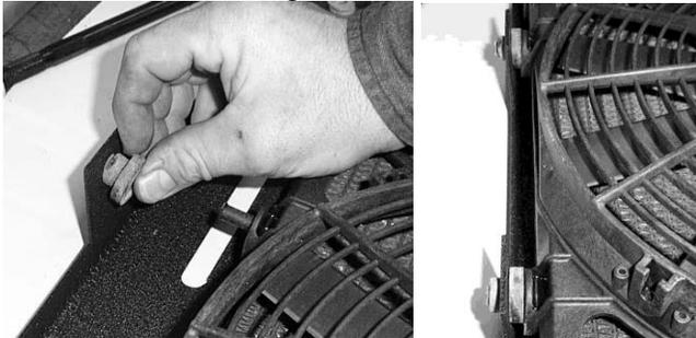
8. Attach the radiator to the kit. Insert the  $\frac{1}{4}$  x  $3\frac{1}{2}$  carriage bolts through the top of the face plate. Place the two long spacers onto the bolt. (In the photo the spacers are square, but were changed to round). Next place the radiator onto the bolts and spacers, then fasten the radiator with the  $\frac{1}{4}$  flat washers and  $\frac{1}{4}$  lock nuts.
