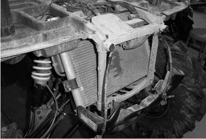
2. Drain the stock radiator and dispose of used fluid according to your local regulations. Use care in disposal, antifreeze is toxic.
