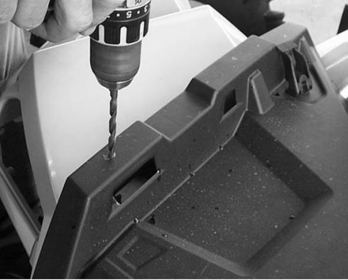
7. Disconnect the front rack from the ATV and cut the holes in the plastic rack and the front plastic fender for hose access.
