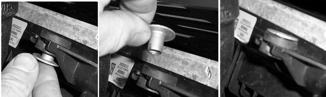
17. Attach the radiator to the kit. Insert the  $\frac{1}{4}$  x  $3\frac{1}{2}$  carriage bolts through the top of the face plate. Place the two long spacers onto the bolts. Next place the radiator onto the bolts and spacers, then fasten the radiator with the  $\frac{1}{4}$  flat washers and  $\frac{1}{4}$  lock nuts.
