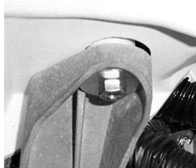
15. The bottom of the stock radiator has two rubber grommets that you will need to place in the holes at the base of the new face plate. Once they are installed insert the bottom of the radiator into the grommets.
