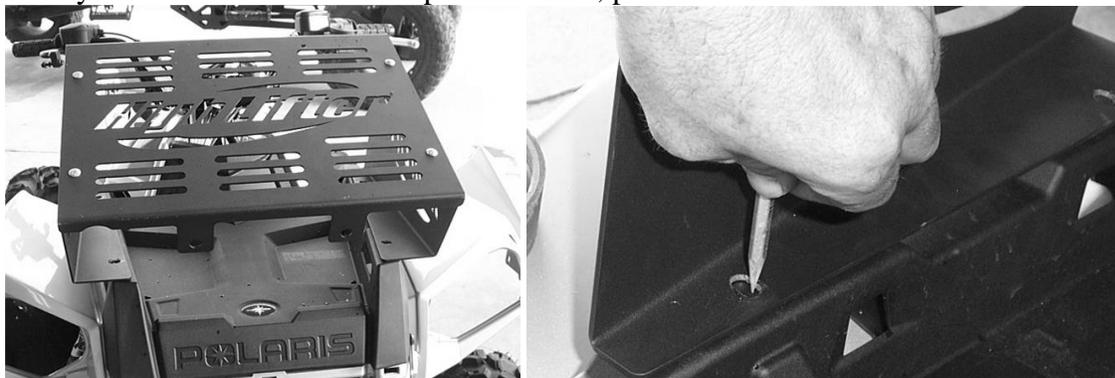
6. Drill out the marked location for attaching the kit to the front plastic rack.
