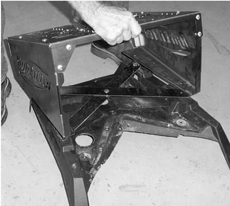
11. Use the  $\frac{1}{4}$ " x 1" bolts,  $\frac{1}{4}$ " washers, and  $\frac{1}{4}$ " lock nuts provided. Place a  $\frac{1}{4}$ " washer on the top in the bolt hole then insert the  $\frac{1}{4}$ " x 1" bolt through the washer and bolt hole. On the underside of the rack place a  $\frac{1}{4}$ " washer on the bolt and secure it using the  $\frac{1}{4}$ " lock nut.
