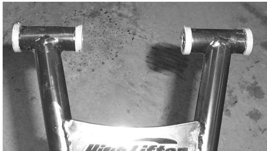
6. Use the factory nuts and bolts to connect the new lower arching A-arms to the UTV. Reconnect the shock to the upper control arm.
