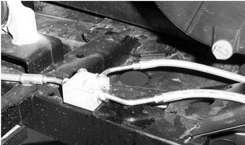
14. Disconnect the brake lines from the junction fitting. Connect the new extension to the brake lines at this time.
