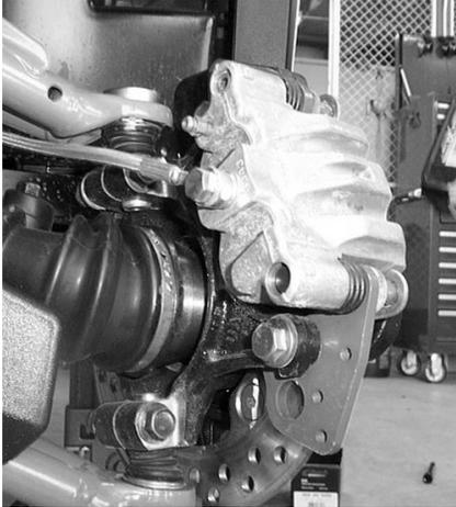
4. Remove the cotter pin and castle nut that secure the brake rotor and axle to the hub assembly.
