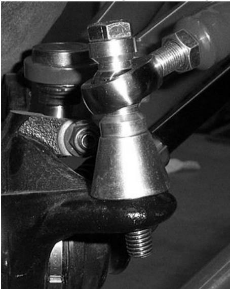
56. Place the ½" washer and ½" lock nut on the bolt and torque tight.
