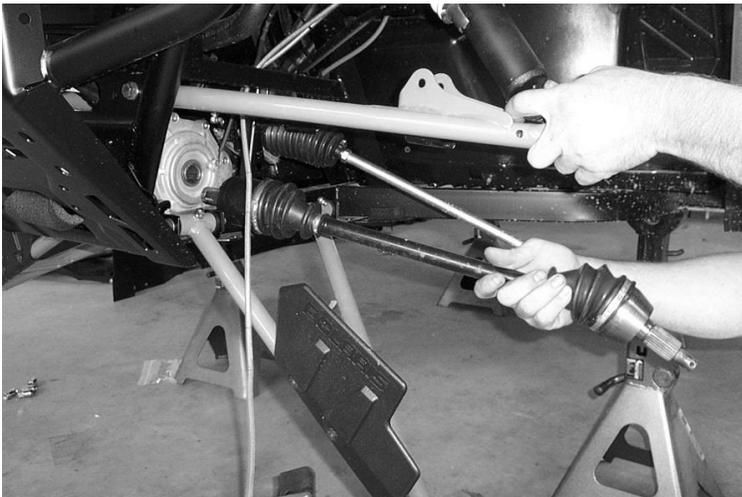
8. Disconnect the tie rods from the rack and pinion. Make sure to leave the factory jam nut in place on the rack and pinion ends.
