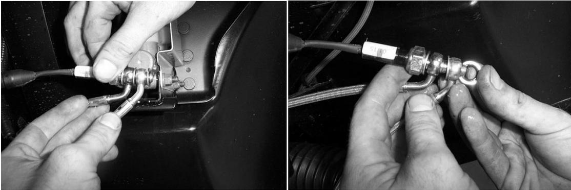
25. Now install the new longer line on the right side of the UTV. Connect it to the master cylinder using the factory hardware.
