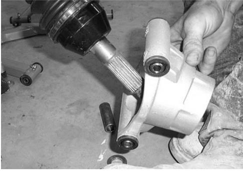
29. Connect the upper arm to the hub assembly using the factory hardware.
