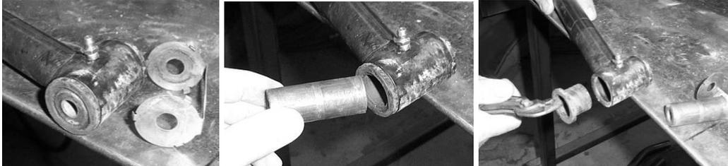
5. Install the grease fitting into the new arms before installation. Install the fittings in the new arms like they are in the factory arms. **DO NOT OVER TORQUE THE FITTINGS.** Make sure to fill with factory approved grease.
