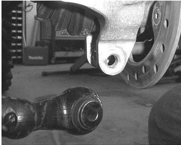
4. Remove the bushings, sleeves, and wear plate from the stock control arms. You will need to reuse these in the new Control Arm kit.
