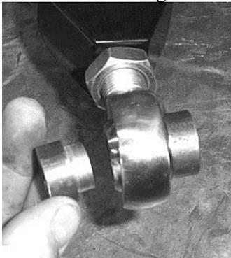
9. Use the factory nuts and bolts to connect the new Control Arms to the RUV frame and knuckle assembly. You will have left and right lower Control Arms. Left and right are determined from the seated position.
