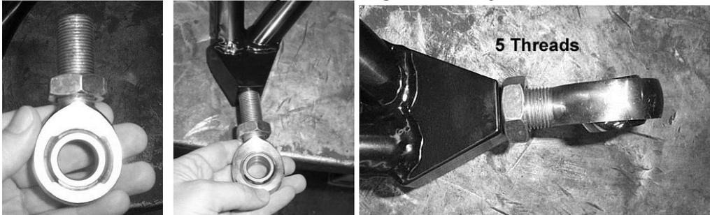
8. Insert the new alignment bushings into the eyelet of the heim joint.
