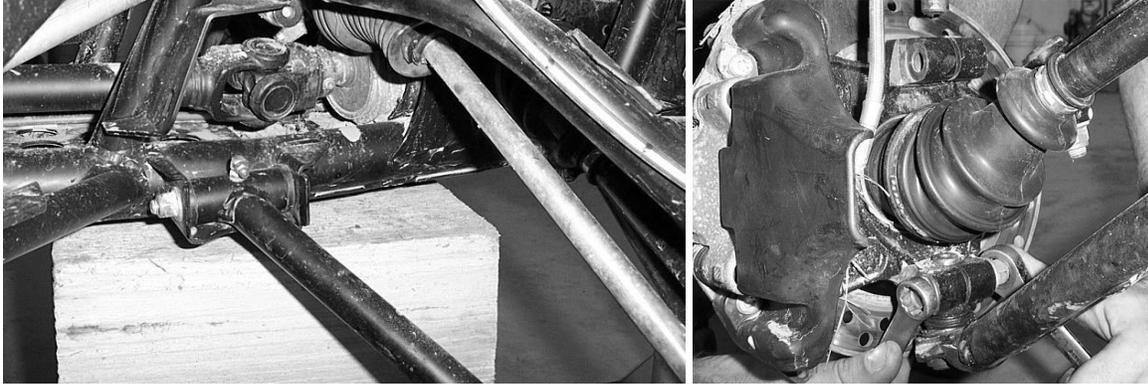
4. Remove the ball joints from the stock control arm. You will need to reuse these in the new kit.
