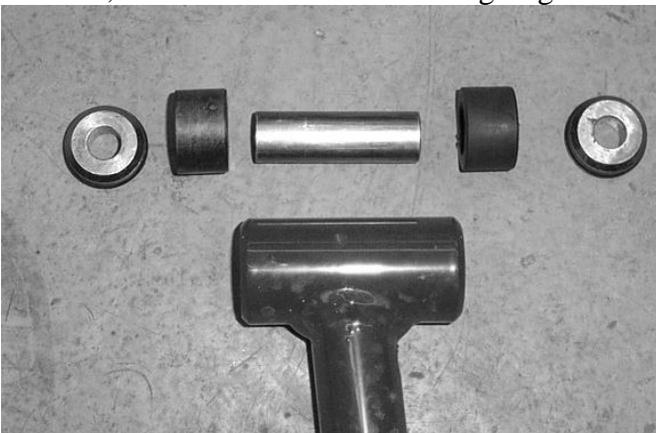
6. Now reinstall the bushings, sleeves, and ball joints into the new arms. If you place some grease on them it makes the installations easier.
