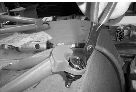
6. Before you install the new control arms you need to install the four steering stops. There are two per side.
