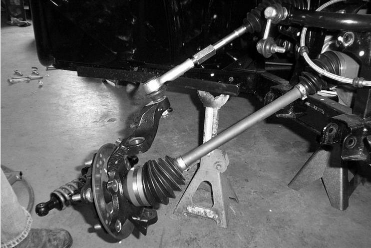
4. Remove the bushings, sleeves, and ball joints from the stock control arms. You will need to reuse these in the new kit.
