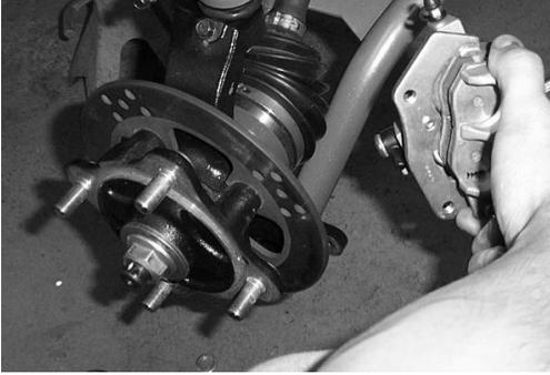
3. Remove the upper and lower control arms from the RUV. Disconnect from the frame, shock, sway-bar, and hub assembly. **NOTE: You do not need to remove the tie rod from the hub.**
