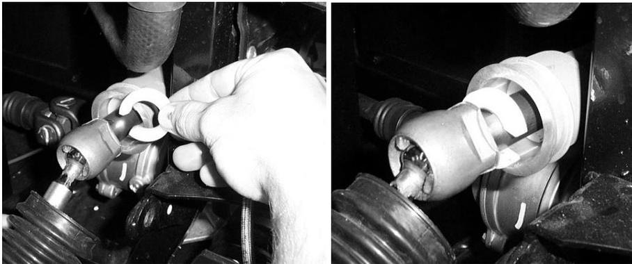
10. Pull boot back over the ball joint and steering stop and refasten with 11" zip tie. Be sure to verify the zip tie is tight so prevent material from getting into the boot.
