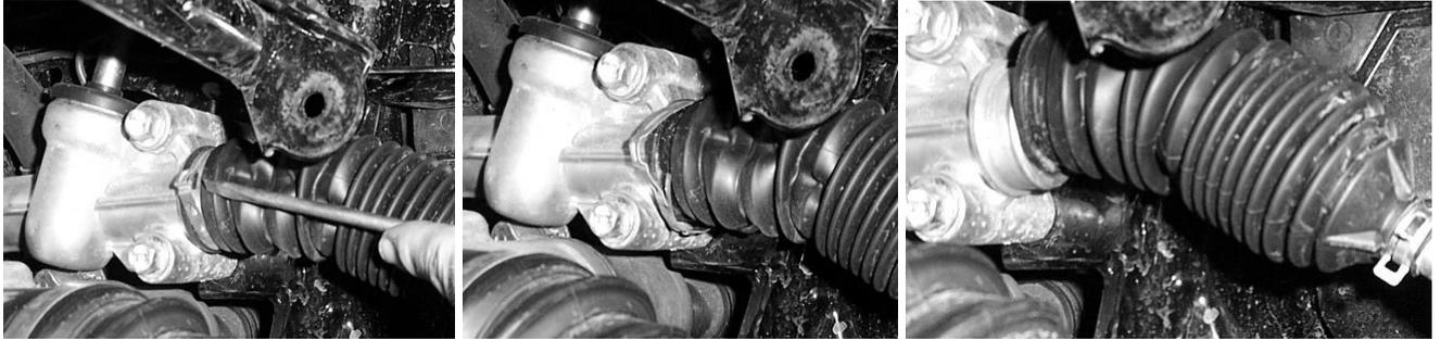
19. Next pull the boot back to expose the inner tie rod joint.
