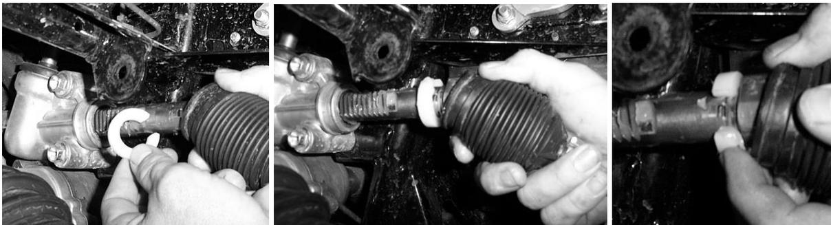
21. Pull boot back over the ball joint and steering stop and refasten with 8" zip tie provided. Be sure to verify the zip tie is tight so prevent material from getting into the boot.
