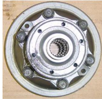
3. Remove the six bolts, then place the differential assembly with the housing side down, and remove the ring gear.
