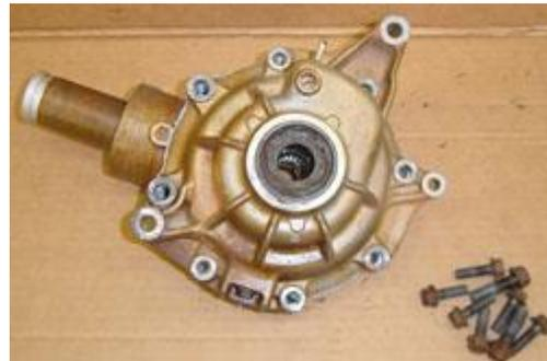
2. Carefully pry the cover off the case using a screwdriver at the pry points, and remove the differential assembly from the differential case.
