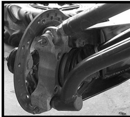
12. Next attached the factory sway bar link to the new trailing arm using the **10x60mm bolt** and **10mm lock nut** provided. Make sure it attaches to the inside of the trailing arm.
