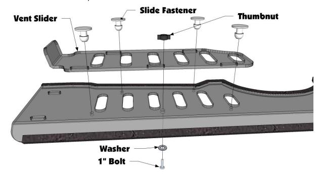
5. When installed the vent should look like the image below.
