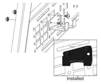
Align holes in the bracket to the holes in the side panel. Insert M8 x 1.25 x 16mm bolts though the holes & securely fasten with the M8 locknut. Repeat on the opposite.
