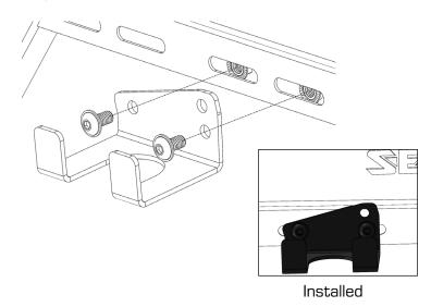
Align holes in the bracket to the slots in the side panel. Insert M8 x 1.25 x 16mm bolts though the holes & securely fasten with the M8 locknut. Repeat on the opposite.
