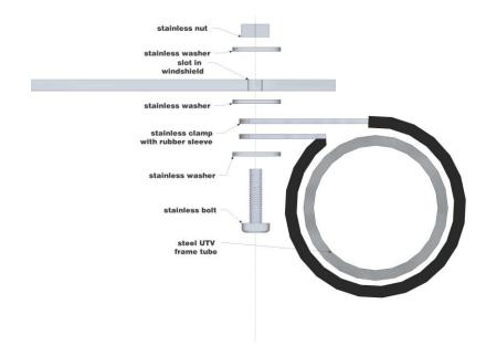
6. Finally install a clamp around the tube blow the hinge as shown below. You will use the 1 1/4" bolts here. This clamp holds the bottom of the windshield down.
