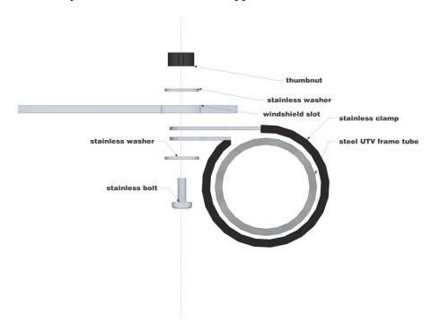
5. Now install the clamp for the slot right above the hinge. You will use the 1 ¼" bolts for this. Below is the diagram showing how this is installed. You will have some of the bolt sticking out towards the front of the vehicle. This is to hold the bottom section of the windshield when it is in the raised position. You will use the same thumb nut for the raised and lowered positions.
