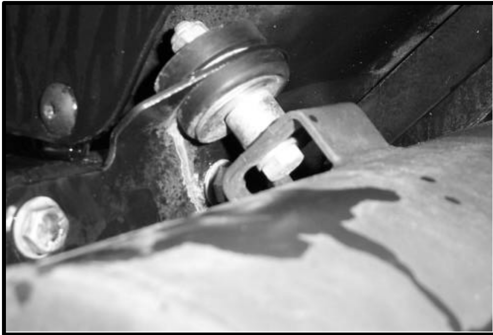
REAR LIFT (BRACKET "G") INSTALLATION PICTURE
